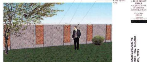
FENCE TYPE #2 6'-0" HIGH MASONRY FENCE PROPOSED APDG A FULL DESIGN GROUP ARCHITECTURE INTERIORS CONSTRUCTION 975.750.4400 WWW.APDG.COM NOTE: REFER TO ARCHITECT
