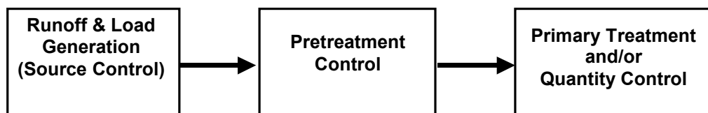
Figure 1.6 Generalized Stormwater Treatment Train
